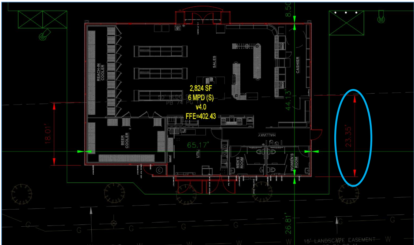
Figure 2: Building Location Encroachment of 23.35ft into the Front Setback Along Goodman Rd
