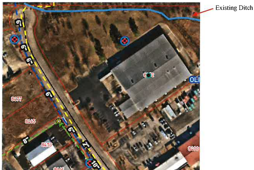
Figure 5: Existing Utilities and Drainage
