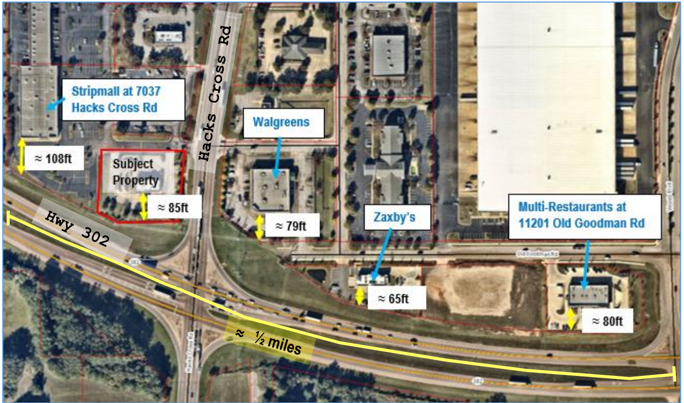
Figure 2: Setback Character of Buildings within Over a Half Mile in the Vicinity of the Subject Property
